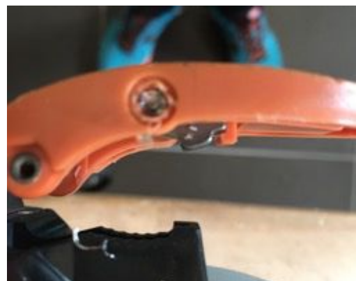
The riveting remove by drilling
